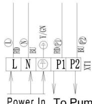
Power In To Pump, Maximum : 250W AC:220V~240V / 50 Hz AC: 220V~240V / 50 Hz
