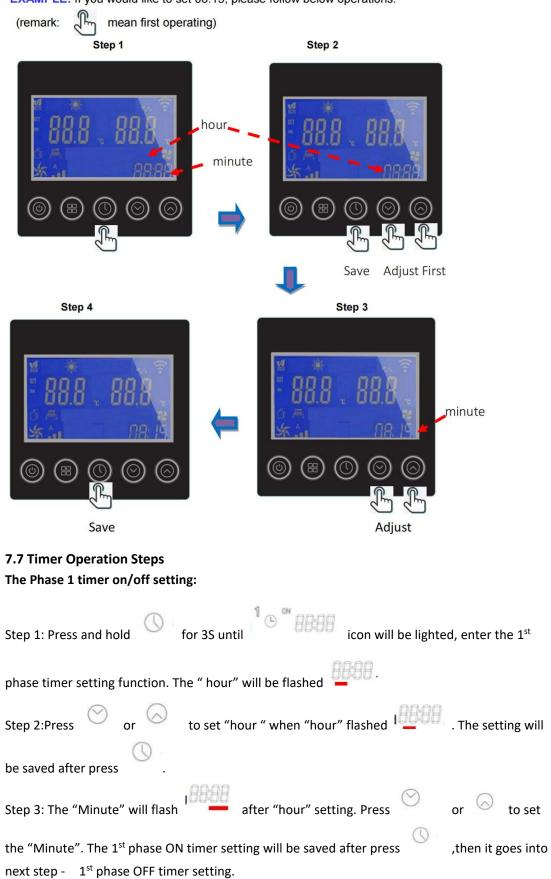
Step 4: 1 C at 8888 icon will be lighted after Step 3 finished, the 1<sup>st</sup> phase OFF timer setting
