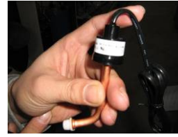
Figure 43: Low pressure sensor.
