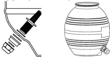
3. Press and turn the sand tank to mount it to sand filter support with correct direction (drain plug is at outside as below picture).
