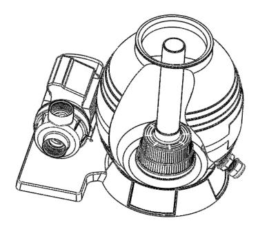
4. Insert the tube with the diffuser body inside the tank as above picture, then place the funnel on the tank's mouth and pour the quartz sand into the tank (sand weight 19kg).
